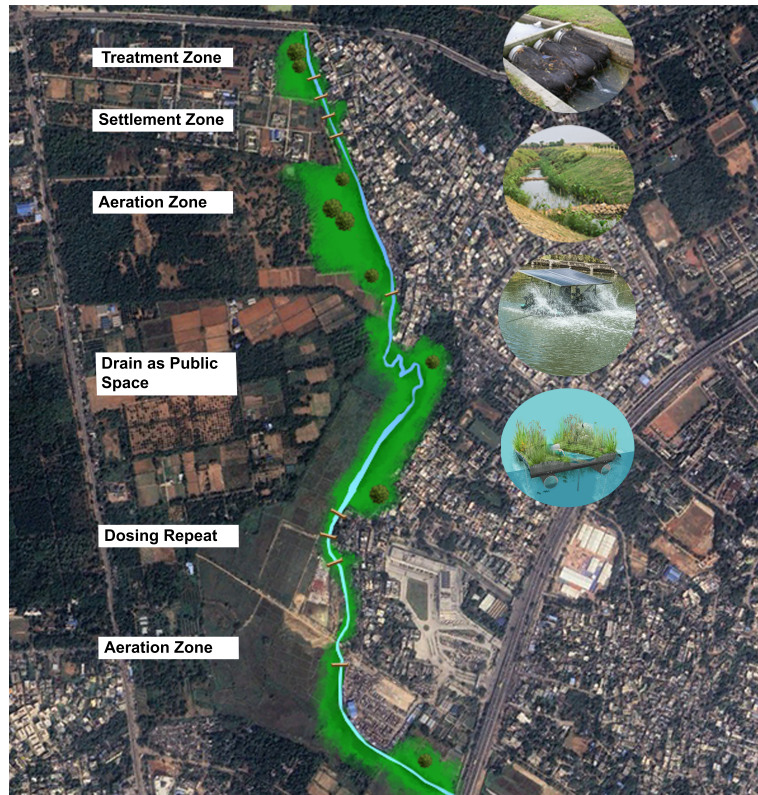
Schematic showing the treatment zone created in the drain 8 for reducing the pollution load from the drain
