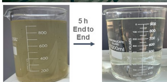
Treatment of Sewage in 10 KLD TADOX based wastewater treatment plant in TERI Gurugram Campus
