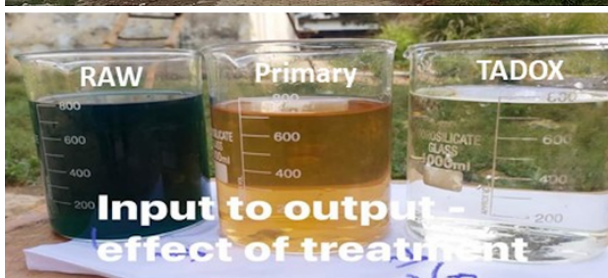
Treatment of Textile wastewater in 20 KLD TADOX based wastewater treatment plant in Kanpur
