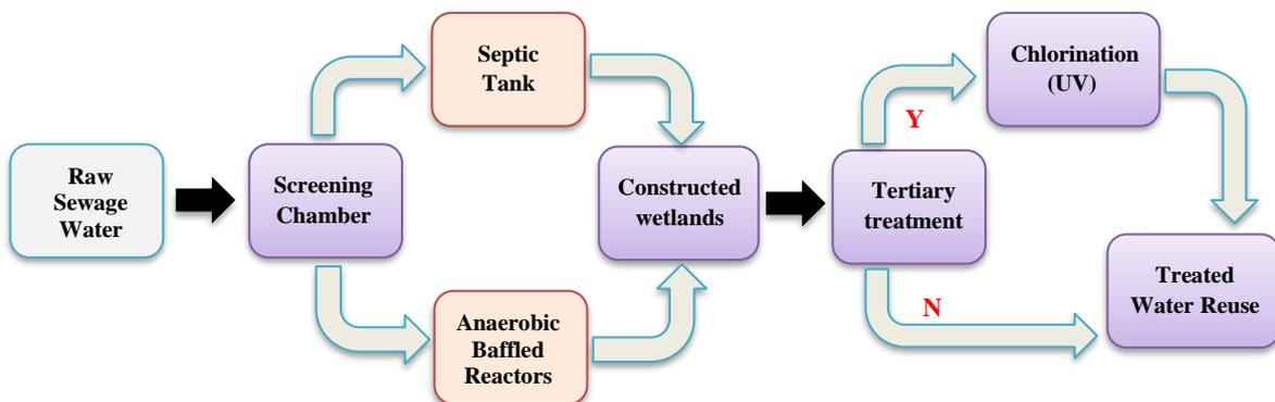
**Figure 11:** Integrated treatment set up with CWs
