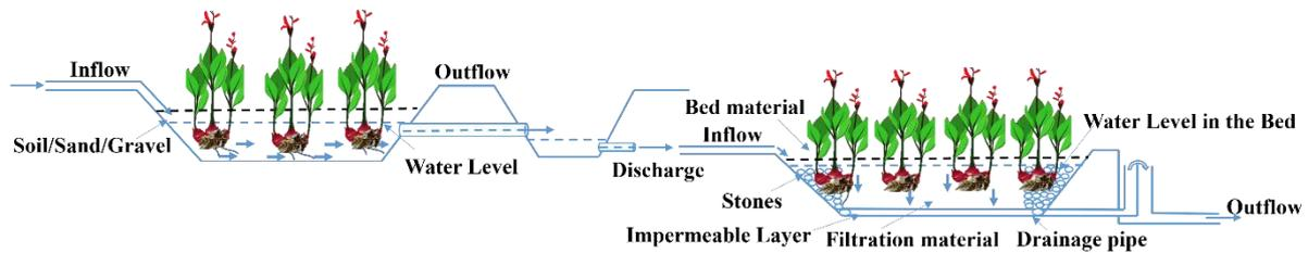
**Figure 5:** Basic design configuration of hybrid constructed wetlands
