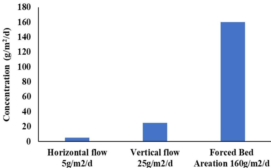
**Figure 12:** Comparison of oxygen transfer rates in CWs
