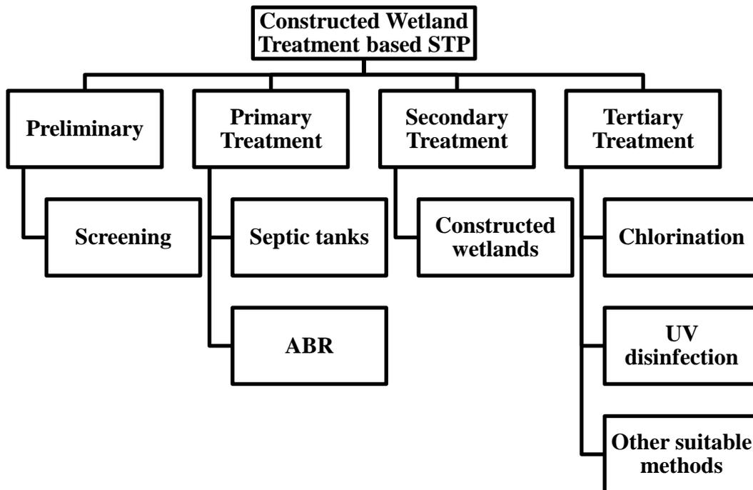
**Figure 9:** Process flow of CWs based STPs
