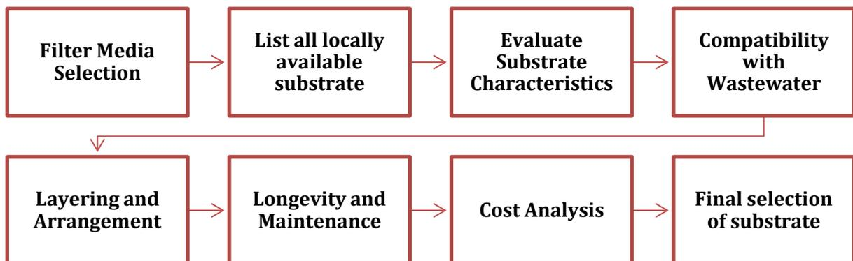
**Figure 13:** Indicative steps for substrate selection for constructed wetlands
